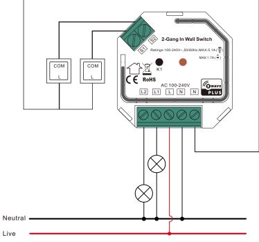
2. Wiring Method 2: External Switches Control through Live Lead 2.1. With 1PC 2-Gang 1-Way Switches
